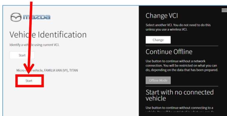
4. Automatic identification is started. If the vehicle is a non-MDARS compliant model, IDS will start up. Please refer to the MDARS User's Guide for details such as when a vehicle cannot be identified.
